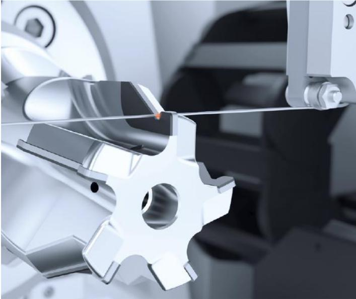
**Caption:** The wire in the VOLLMER VPulse 500 wire erosion machine is guided close to the workpiece until a spark is generated and removes the PCD material.
